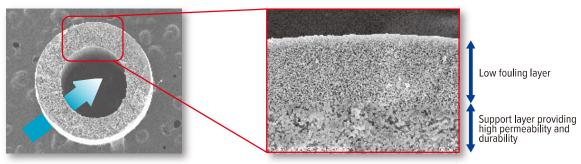
Outside-In flow direction is ideal for treating water with high turbidity. Suspended solids are effectively removed during backwash and air scouring.
